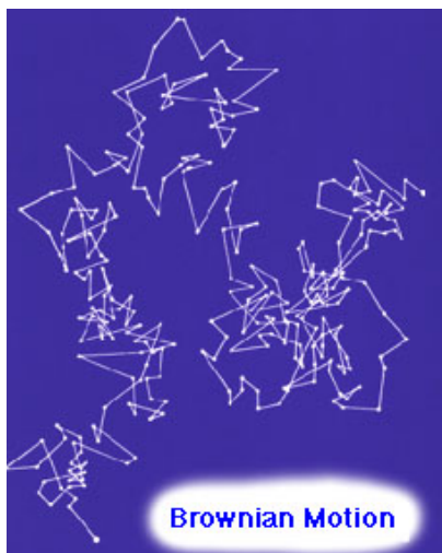
Figure 1 shows the position at 30 second intervals of a 0.53 micron particle in water as observed by Perrin under a microscope. (From Mandelbrot, Fractals , 1983)
